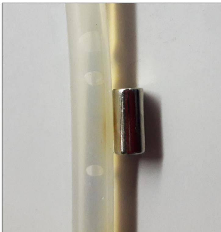
Figure 2. The magnet is able to stop the  $^{Fe}CaPs$  from following the fluid flow with the capillary velocity.
