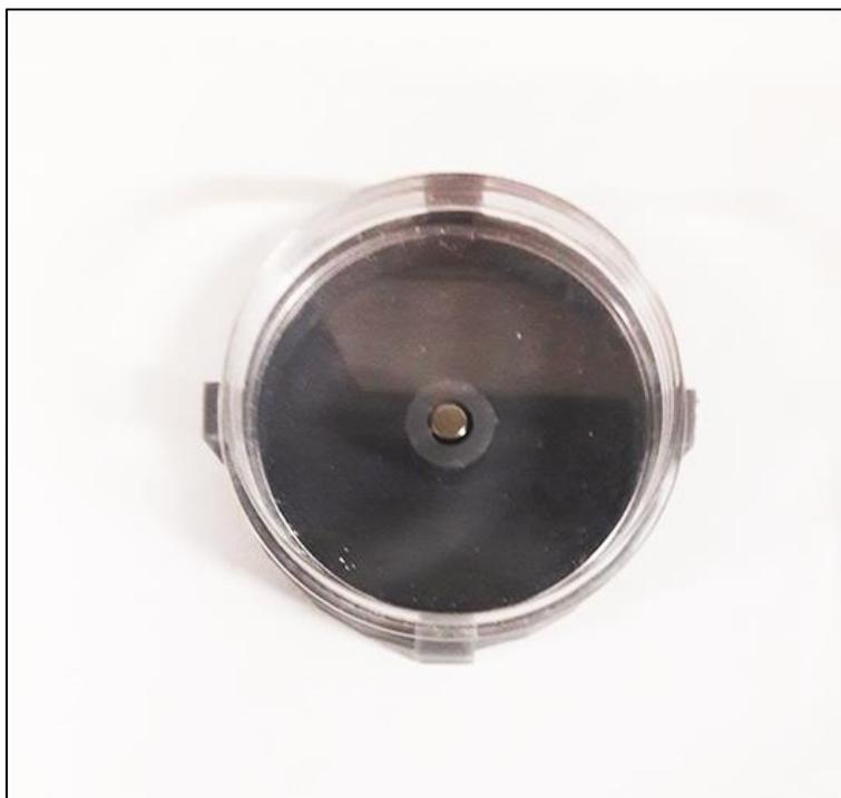
Figure 6. 3D printed support to place the magnet below a petri dishes where to perform cell culture tests.
