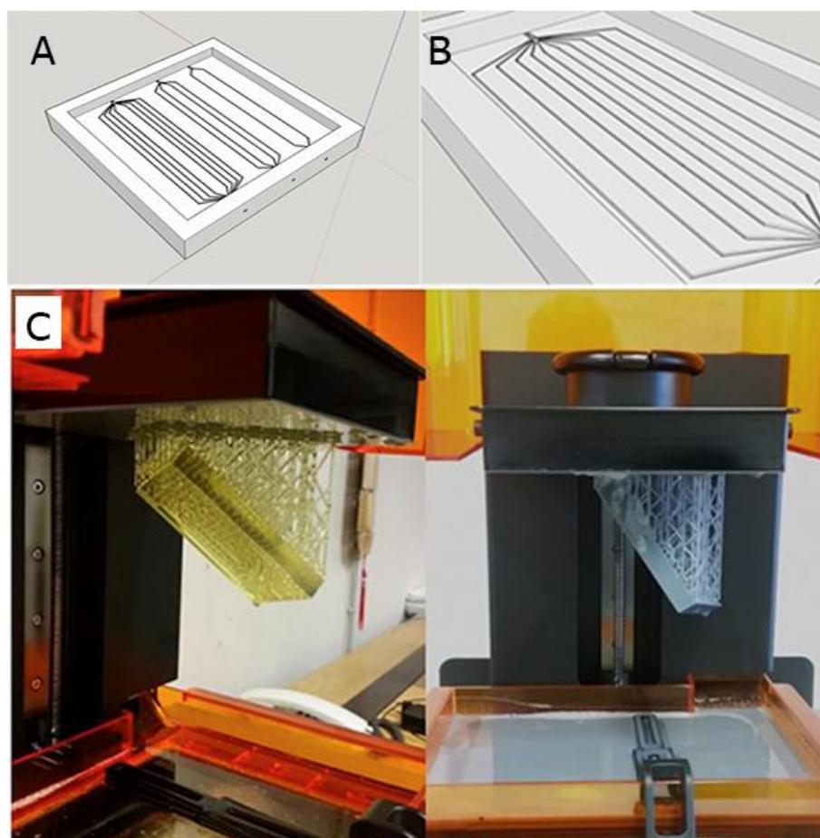
Figure 3. Different phases of the stereolithography 3D printing procedures of the micro-fluidic device. Panels A, B represent the CAD sketches (realized through the Sketchup software (Version 2016)). Panel C shows the device during printing phase.
